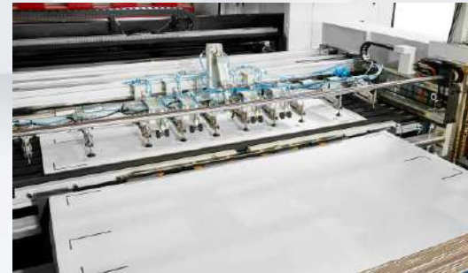
Fully automatic top feeder module working with the production line.
